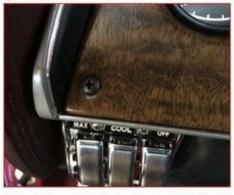
2. The plastic parts of the dash can become fairly brittle with age, so easy does it. The trip odometer reset button unscrews, and the wiper switch knob has a set screw on the bottom. (The 1967 wiper knob is thinner and it doesn't need to be removed.) These must be removed before the instruments can be removed from the bezel.
