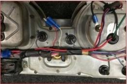
6. You will need to run a new wire through the firewall grommet adjacent to the ignition feed wire. You can use a short piece of brass tube to punch the hole for the wire. (In Issue 2 we demonstrate the technique.) Run the wire to the coil negative post.
