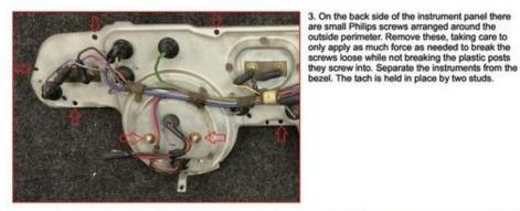
The new tach mounts in exactly the same way as the old one. We chose to upgrade to the 8K RPM version.
